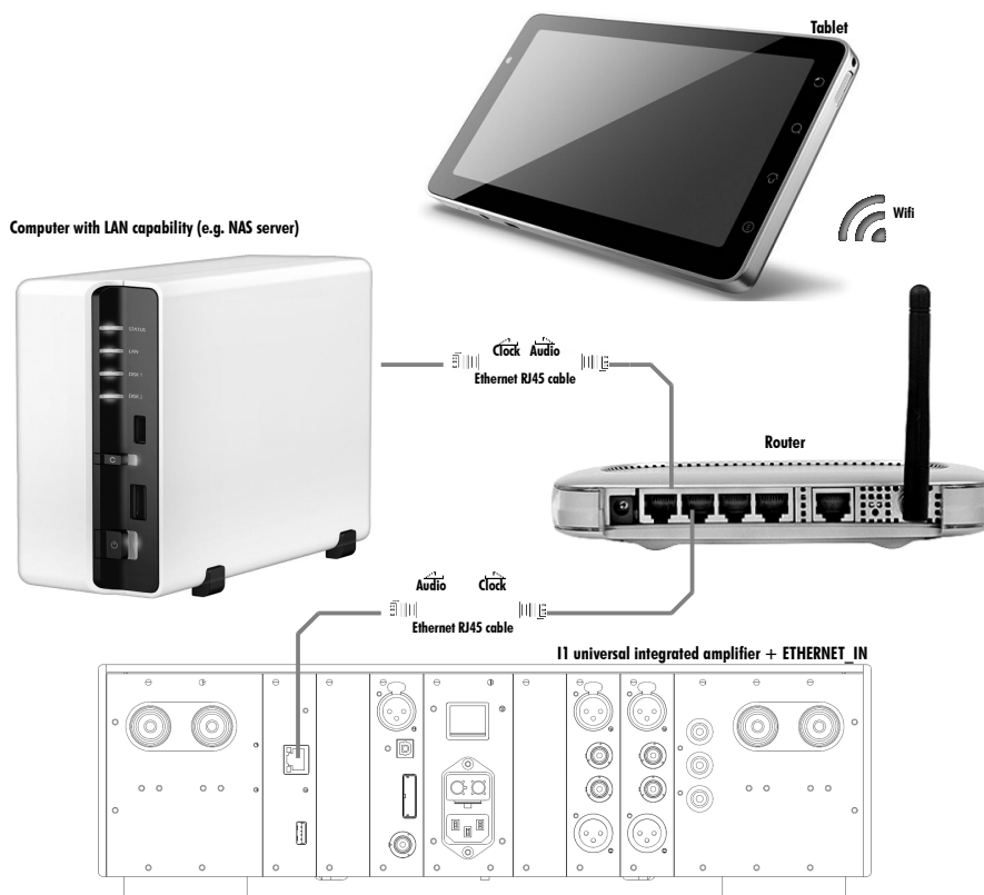
Computer to I1 with ETHERNET_IN board
