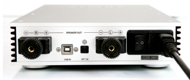
Figure 6. AC Power Cable Connection
