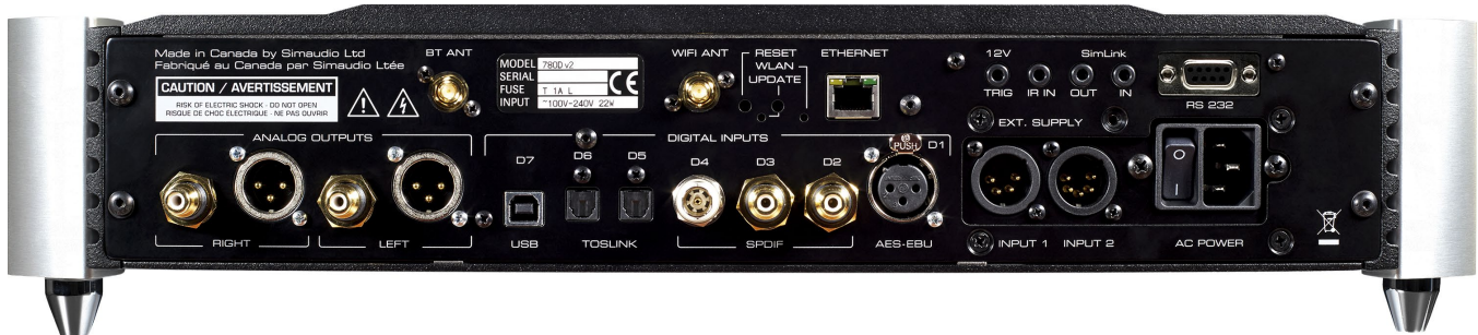
Figure 2: 780D v2 Rear panel
