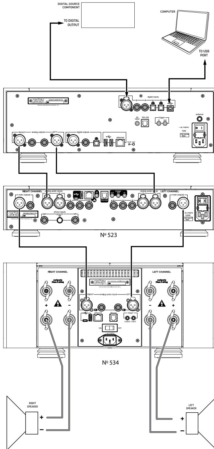
Nº 519 connected to a preamp using the digital outputs
