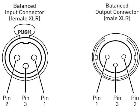
**Digital output connectors:** the № 519 has three digital output connectors: AES/EBU Balanced XLR, Coaxial S/PDIF RCA, and Optical S/PDIF TOSLINK. Each digital output provides a two-channel digital connection to your DAC or preamplifier with built-in DAC. Mark Levinson recommends using the Balanced digital output for the best possible sound quality if the connection is available on the DAC or preamplifier to which the player is connected.
