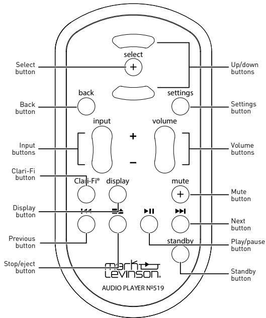
**Standby button:** press this button to put the unit into and out of the selected Standby mode.
