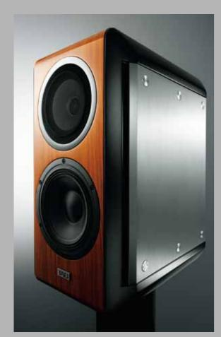
The SILENT\* enclosure brings together TAD's theory and technology. The cornerstones of its outstanding physical properties are its combination of birch plywood braces, MDF panels and Bi-Directional ADS Port featuring 10mm-thick hard anodized aluminum side panels that provide superior strength and vibratio dampening. Additionally, optimization of the enclosure size and port layout have eliminated standing waves up to 250Hz.
