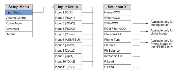
The Input Setup menu allows you to customize the following parameters for the selected input:
