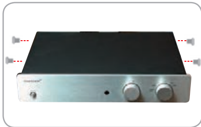
3 Remove the four cover screws.
