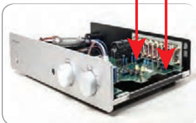
6 Observe the position of the plug on the phono module and carefully plug it in, ensuring that all of the pins are inserted correctly into their connectors.
